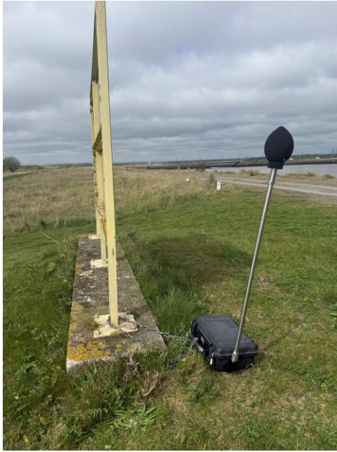
Inset 6.6 Environmental sound measurement setup at location U1
