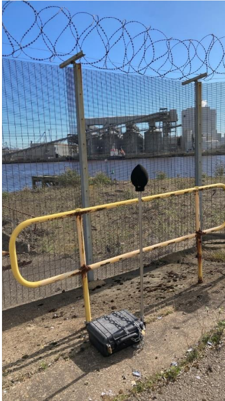
Inset 6.46 Environmental sound and meteorological measurement setup at location U9
