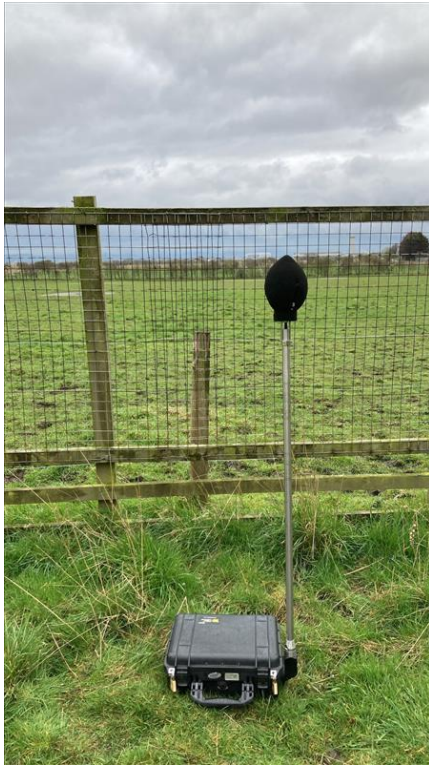
Inset 6.26 Environmental sound measurement setup at location U5
