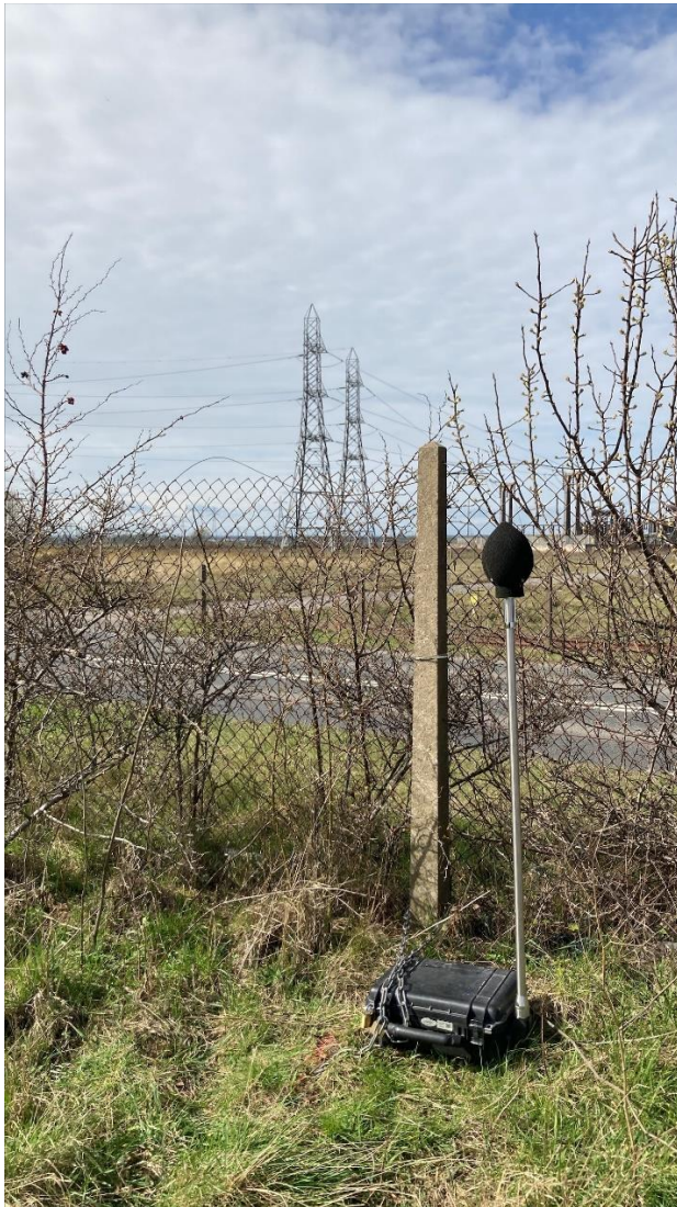
Inset 6.36 Environmental sound measurement setup at location U7
